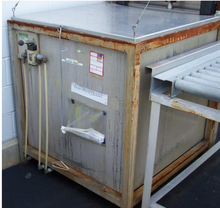
Penetrant Station with Power Immersion Grille
