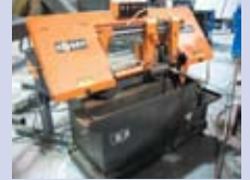
GOSEN Mdl M H - 1016JA, 2 HP Horizontal Band Saw w/Coolant Feed, S/N 94106219, Mfg. 2008
