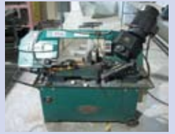
Central Machinery Horizontal Metal Cutting Band Saw, 4-1/2" Round 4" x 6" Rect Cap
