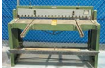
Central 52" Sheet Metal Shear
