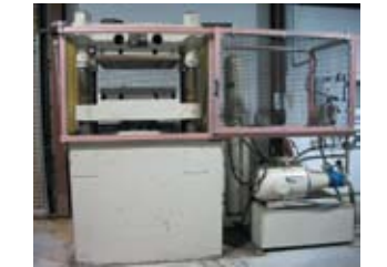
Watson-Stillman Hydro Forming Press 77-231 Ton, 30" x 28" Table, Hyd Power Unit w/Manual Controls & Safety Enclosure, 25 HP Motor w/Steel Head, Has Spare Rubber Heads
