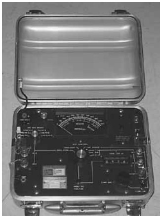
Barfield P/N 101-00164 Pitot Static Test Set
