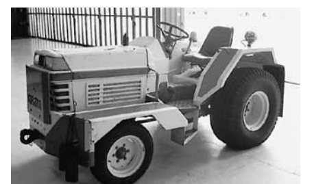
Kubota Aircraft Tug w/Perkins 4-Cylinder Diesel Engine
