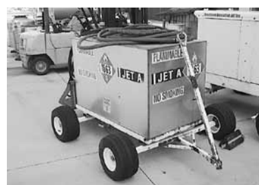
(2) Jet A 275 Gallon Fuel/De-Fuel Carts, Stainless Steel Tank w/Yamada Diaphragm Pump
