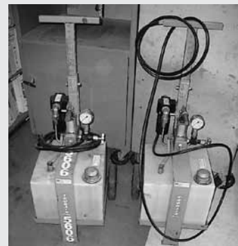
(3) Tronair Mdl 06-4035-0500 Hydraulic Service Units, 8-Gallon Capacity, (2) 83282 Fluid, (1) 5606 Fluid
