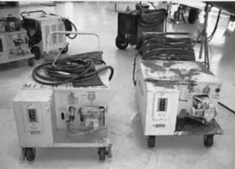
Tronair Mdl 05-7008-3400 Hydraulic Power Unit, Skydrol 500 Fluid, Pressure Range 0-1,750 PSI, Flow Range 0-6 GPM
