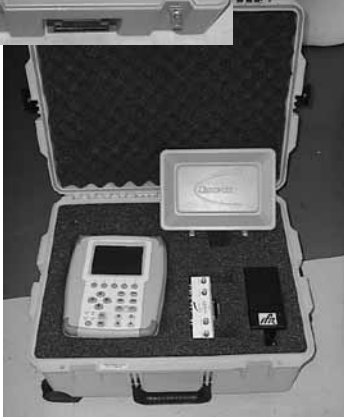
Barfield P/N 101-00164 Pitot Static Test Set
