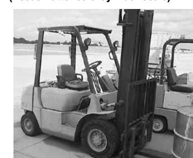
Mitsubishi Mdl FD-25 Forklift, 4,000 LB Gas, Dual Stage 12' Mast, Pneumatic Tires
