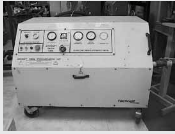
Tronair Mdl 15B7603-1000 Cabin Pressurization Unit, Pressure Range 0-13 PSI, Flow Range 0-275 SCFM
