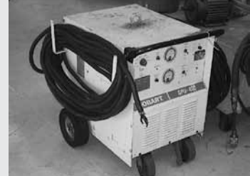
Hobart GPU-400 GPU, 28 Volts, 400 Amp
