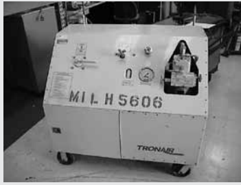
Tronair Mdl 05-3010-1100, 81 Hydraulic Power Unit, 5606 Fluid, Pressure Range 250-3,000 PSI, Flow Range 0-10 GPM
