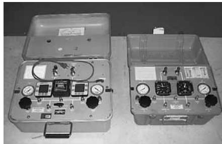
Barfield P/N 101-00164 Pitot Static Test Set
