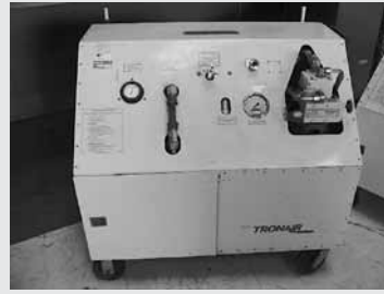
Tronair Mdl 5B200ATI Hydraulic Power Unit, Fluid MIL-PRF-83282D, Pressure Range 250-3,000 PSI, Flow Range 0-6 GPM
