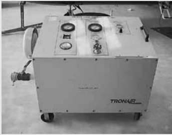
Tronair Mdl 15-7602-1000-81 Cabin Pressurization Unit, 15 HP Motor, Pressure Range 1-12 PSIG, Air Flow 0-240 ACFM
