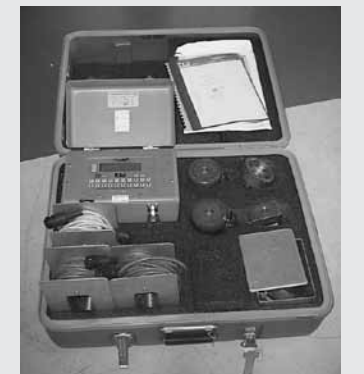
Evergreen Roadrunner III Electronic Aircraft Scales w/Jack Point Load Cells, (2) 20,000 LB & Full Function Indicator P/N 3-0101-299C, For Helicopters & Small Fixed Wing Aircraft
