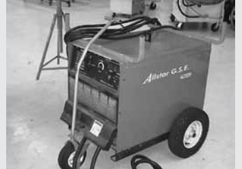
(2) Allstar GSE Mdl AL2000R/RT Aircraft Ground Power Units (Rectifiers), Input 230/460/575 Volt, 96/48/38 Amps, 34.2 KW, 60 Hz, 3-Phase, Output 44 Volts, 650 Amps, 100% Duty Cycle
