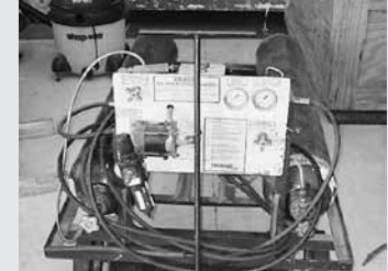
Tronair Mdl 5B200ATI Hydraulic Power Unit, Fluid MIL-PRF-83282D, Pressure Range 250-3,000 PSI, Flow Range 0-6 GPM
