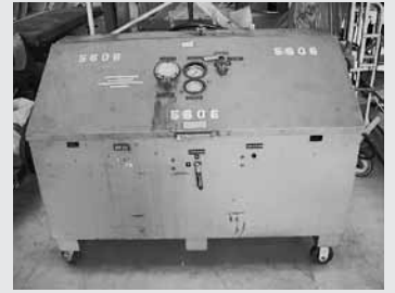
Titan Aerospace Mdl GS-3000-10RC Hydraulic Power Unit, Pressure Range 250-3,000 PSI, Flow Range 0-10 GPM, Fluid MIL-H-5606
