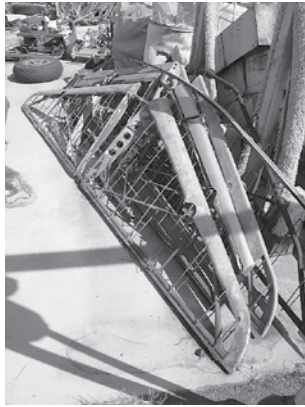
(17) Stearman Elevator Cores
