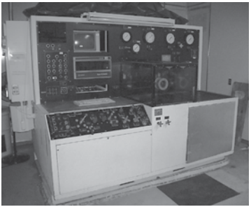
American Lab & Systems Mdl. 86AP198 Hydraulic Pump Motor Test Bench, S/N 147, 5606 Fluid, Dual 50hp Motor & Pumps, Hydraulic Driven Single Pad Drive, Digital & Analog Pressure and Flow Meters, 10-15,000 RPM, 3500 PSI, 20 GPM, Computer Display Flow Meter, Mfd. 11-17-89
