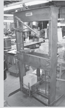
Dake Mdl. 50 HW 5 Ton H Frame Hyd. Press Small Hyd. H Frame Press Essick Mdl. F-390 Horizontal Aircompressor Dual Stage
