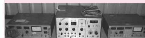
MEC-720 A Transponder Test Set MEC-820 DME Test Set MEC-730 Ramp Transponder Test Set
