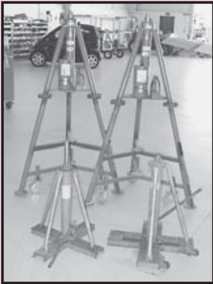
(2 Ea.) Tronair Mdl. #02-0566-0100, 5 Ton 24" Aircraft Jacks w/Stands to Make High Wings (3 Ea.) Jack House, 30" Jacks (2 Ea.) 24" Aircraft Jacks
