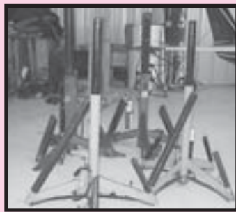
(2 Ea.) Meyers 36" 3-Ton Aircraft Jacks w/Extensions (2 Ea.) Ward Aero 36" 3-Ton Aircraft Jacks w/Extensions P/N 2-170
