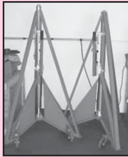
Shop Built 3-Ton High Wing Jacks (3 Ea.) Tail Stands D & C Mdl. #DE-201 Nicad Battery Charger/Discharger
