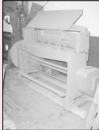
Wysong & Miles No. 552 Shearmaster, 52" Power Shear
