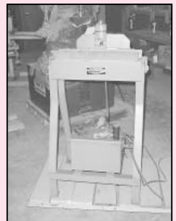
Lockformer Button Punch & Cheek Bender, 22", 20 Ga. w/ Notcher
