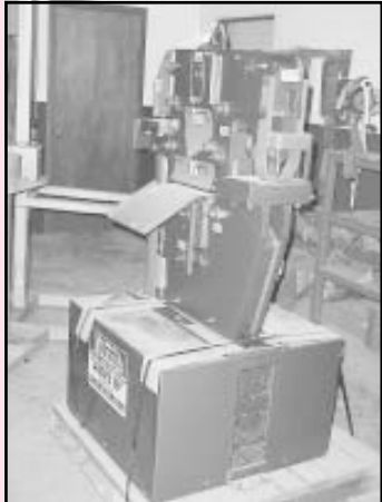
Edwards Mdl. 1W-5, Jaws IV Ironworker, 50 Ton Punch 7" Throat, Bar Shear 3/4" x 4" Flat Thickness, 1/2" x 10" Flat, Angle Shear 4" x 4" x 1/4", Notching 5/16" x 2" x 3"
