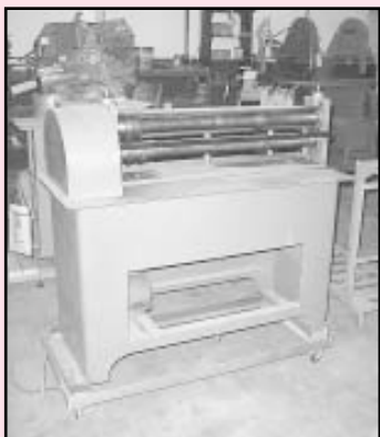
Flagler Mdl. GSL 36" Gang Slitter, 22 Ga.
