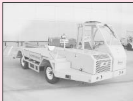
(3 Ea.) Accessory Controls & Equip. Mdl. 1410RJ-FD Lavatory Service Units, Drive Around, 500 Gal. Waste, 300 Gal. Water, Pumping Cap. 24 G.P.M. @40 P.S.I., 4 Cyl. Gas Ford Engines, Mfg. 2000 and 2001 1980 Ford Lav Truck, 500 Gal. Waste Tank, Auto Trans., V-8
