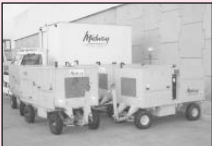
(6 Ea.) Spencer Industries Cold Buster Mark I, Aircraft Heater Carts, Ford 6 Cyl. Engines, Mfg. '98' and 2000
