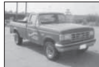
1990 Ford F-150 Custom Pickup, 4.9 Liter Fuel Injected 6 Cyl., 4 Speed Trans. with Overdrive, 4x4
