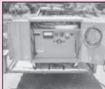
(2 Ea.) Cabin Pressurization Carts, Built by Lock Haven Airmotive, Inc.; Being used on Lear Jets, Citations, Commanders, Etc.
