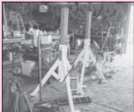
(2 Ea.) Support Systems, Inc., Aircraft Jacks, P.N. 10-013-11, 10,000 Lb., 48 Inch with Extensions
