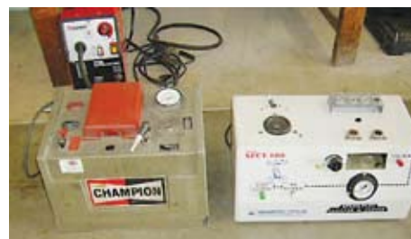
Champion Spark Plug Cleaner/Tester ATS Spark Plug Cleaner/Tester Vixen Spark Plug Cleaner/Tester Champion Spark Plug Vibrator/Cleaner & Gaper
