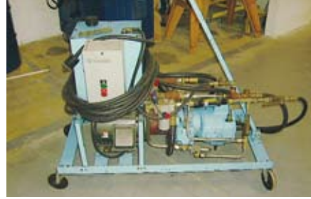
Hydraulic Mule; 3000-5000 PSI; 7 1/2 HP Motor
