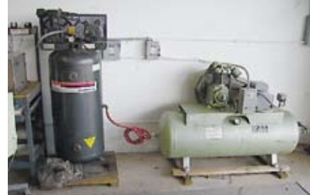
Sanborn Mdl 500B60U Vertical Air Compressor; 5 HP; 1 Single Phase; 2 Stage; 60 Gal Tank
