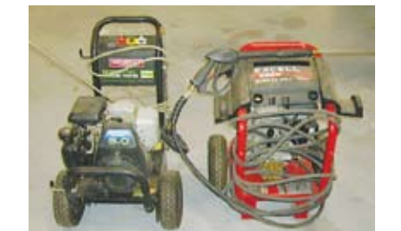
Generac Portable Pressure Washer; 2400 PSI w/Honda 5 HP Gas Engine Excell Portable Pressure Washer; 2800 PSI w/Honda 6 HP Gas Engine
