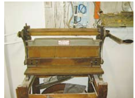
Central Machinery Mdl SKU-T590 Universal Sheet Metal Working Machine; includes 30" Shear; Press; Brake & Slip Roller 36" Sheet Metal Break
