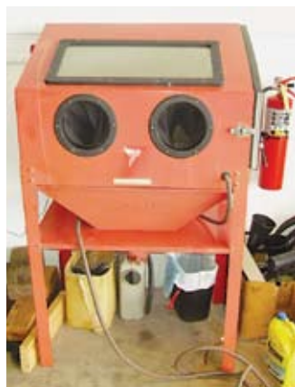
Sand Blast Cabinet; Inside Measurement 36" Wide 22" Deep; 20" Tall
