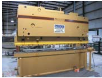
Standard Industrial Corp Mdl AB200-12, 12'/200 Ton Press Brake, 132 Ton Punch Cap w/CNC 150 Auto Gauge, 2-Axles Controller & Back Gauge, Ram Stroke 8", Open Height 14" Max, Closed Height 6" Min, 20 HP Motor, S/N F2061462
