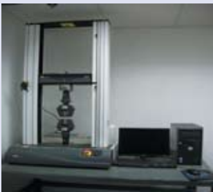
Instron Mdl 3369 Dual Frame Electrical Mechanical Tension/Compression Load Tester w/Instron Computer Software Load Cap 11,240 Lbs, Max Speed 20" Per Minute
